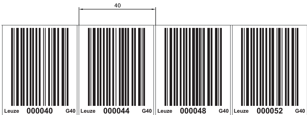
Fig. 9.1: Checking the print result – BCB G40 ...-repair kit (40 mm gird)
