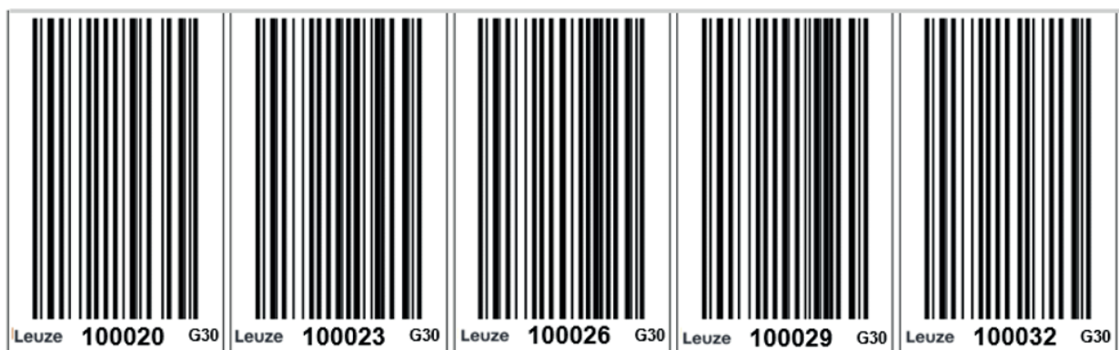
Fig. 3.2: Bar code tape, beginning with position value 1000.20 m, increasing in increments of 3 cm
