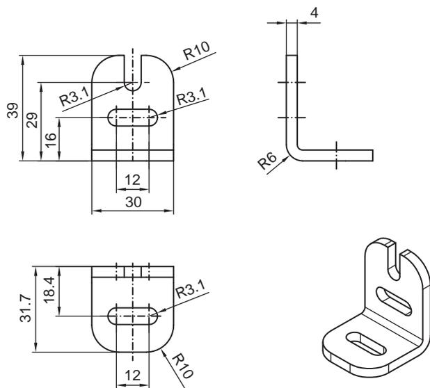
Figura 14.2: Soporte angular BT-L
