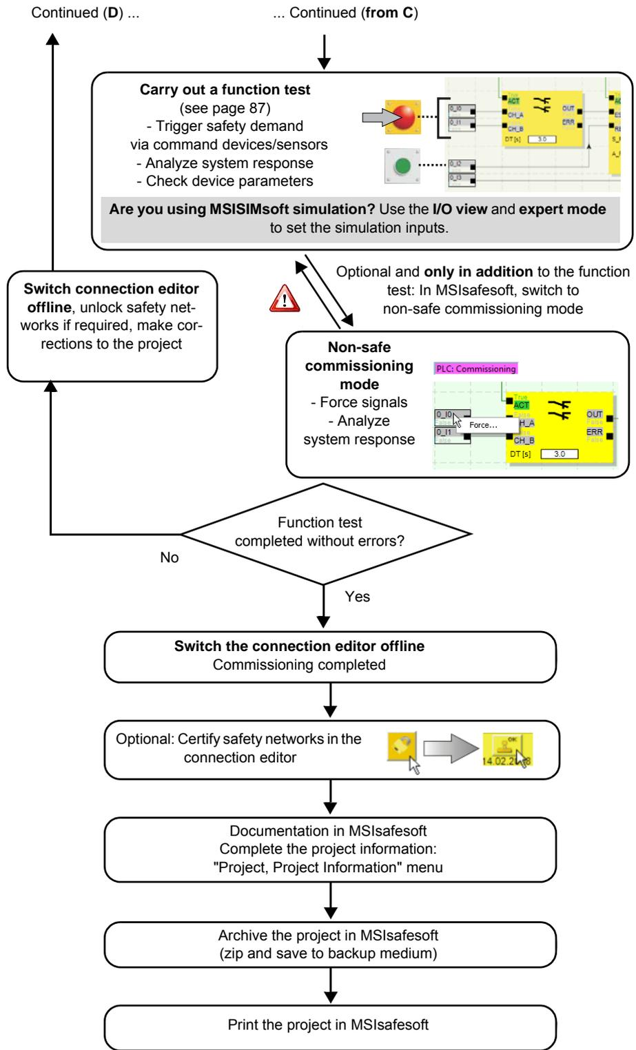
Figure 10-3 Flow chart: Example configuration and commissioning (3 of 3)
