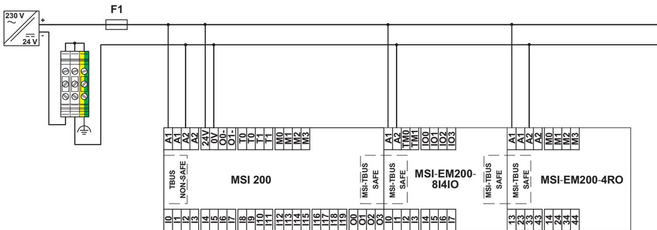
Figure 7-7 MSI 100/200 system voltage supply
