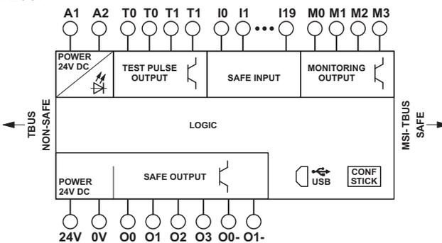
Figure 3-3 MSI 200 block diagram
