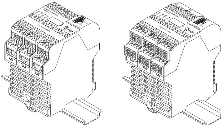
Figure 3-1 Screw terminals (left) and spring-cage terminals (right)
