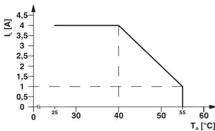
Figure 14-3 Derating curve MSI-EM200-4RO
