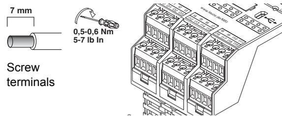
Figure 7-3 Connecting to screw terminals
