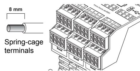
Figure 7-4 Connecting to spring-cage terminals
