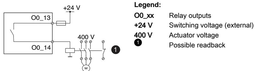
Figure 6-13 Single-channel assignment of the relay outputs
