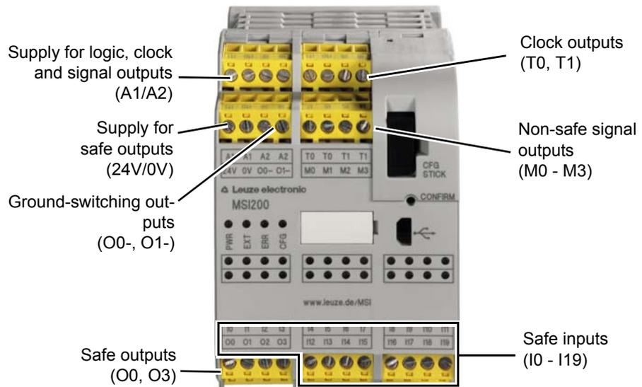
Figure 3-8 Signal connections MSI 100/200
