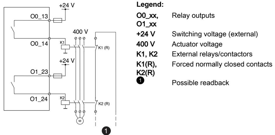
Figure 6-14 Two-channel assignment of the relay outputs
