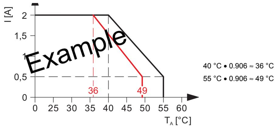
Figure 14-4 Example of a shifted derating curve (red)
