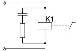
Figure 6-9 Example for the freewheeling circuit of an external relay
