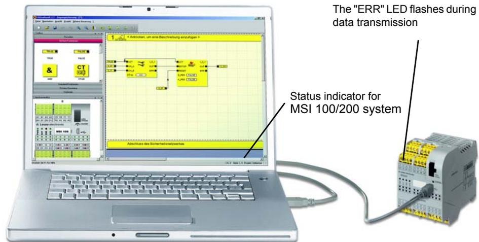
Figure 10-4 USB connection between PC and safety module
