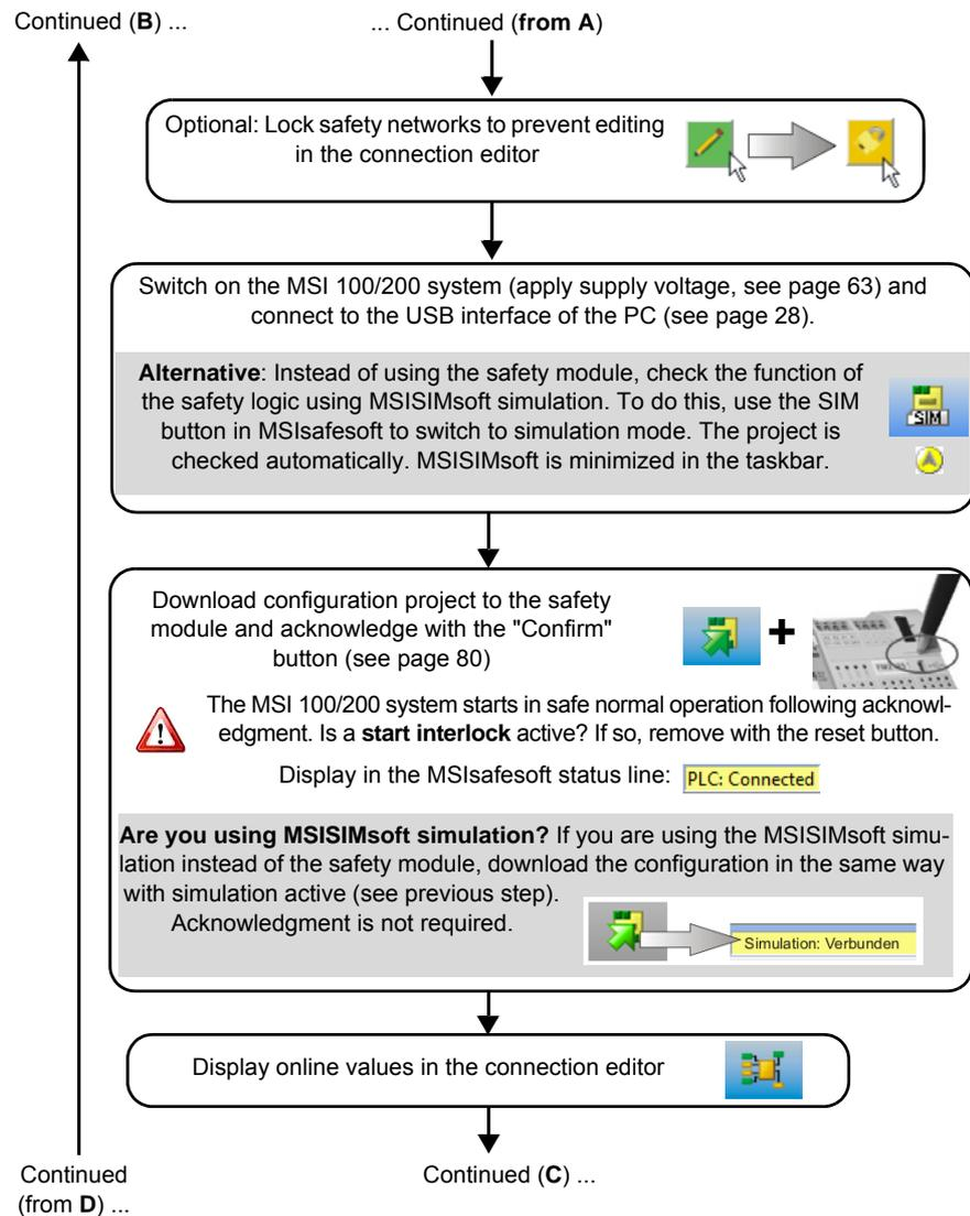
Figure 10-2 Flow chart: Example configuration and commissioning (2 of 3)
