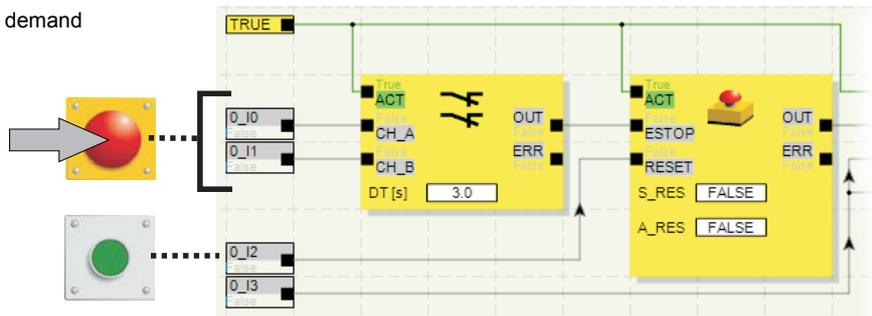
Figure 10-8 Example of a function test for the safety system using the online mode of MSIsafesoft
