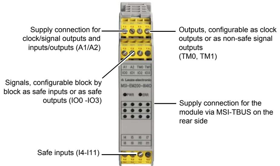
Figure 4-4 Signal connections MSI-EM200-8I4IO
