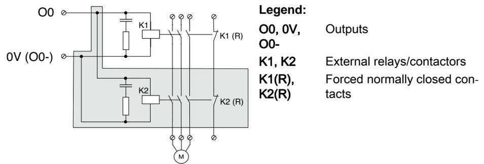
Figure 6-10 Single-channel assignment of the outputs
