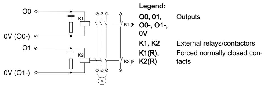
Figure 6-11 Two-channel assignment of the outputs
