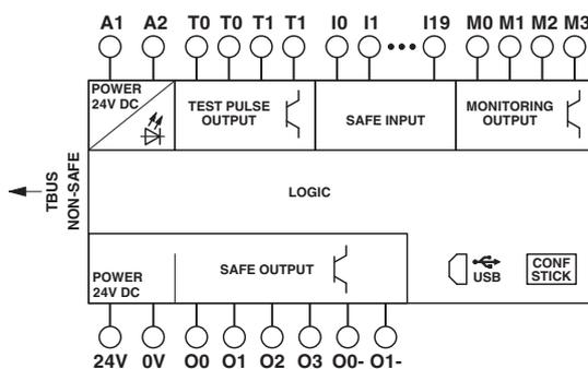
Figure 3-2 MSI 100 block diagram
