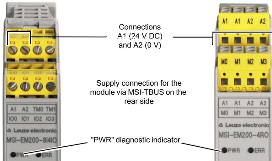
Figure 7-6 Connecting the supply voltage
