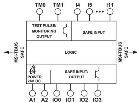
Figure 4-2 MSI-EM200-8I4IO block diagram
