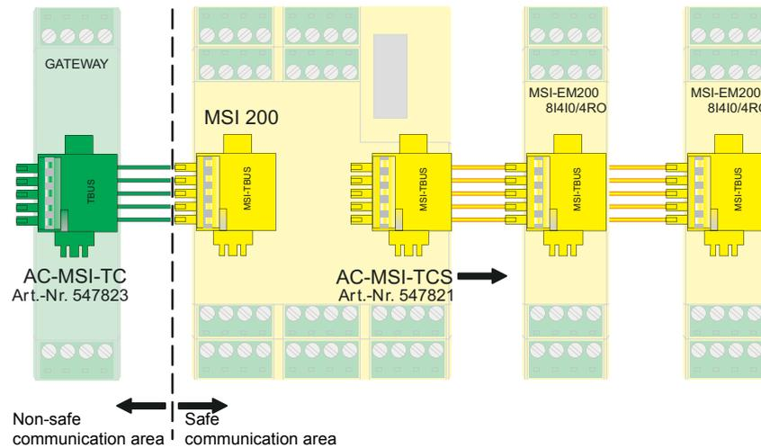
Figure 2-2 Extension of the MSI 200 safety module
