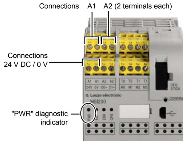
Figure 7-5 Connecting the MSI 100/200 supply voltage
