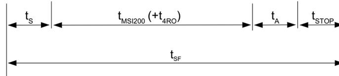
Figure A-1 Switch-off time for the safety function
