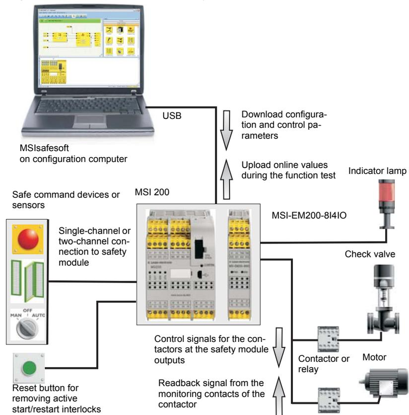
Figure 2-1 Typical structure of a safety system with MSI 200
