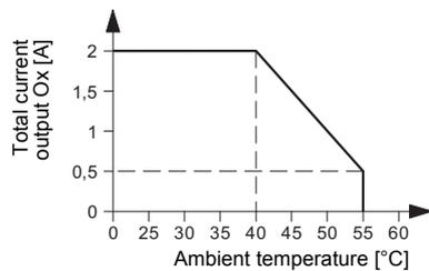
Figure 14-1 Derating curve MSI 100 and MSI 200
