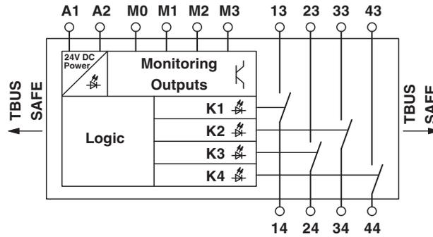
Figure 5-2 MSI-EM200-4RO block diagram
