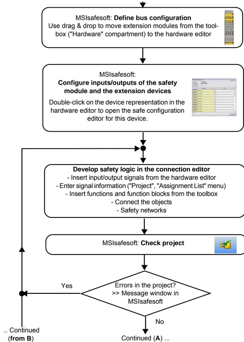
Figure 10-1 Flow chart: Example configuration and commissioning (1 of 3)
