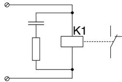
Figure 6-12 Example for the freewheeling circuit of an external relay
