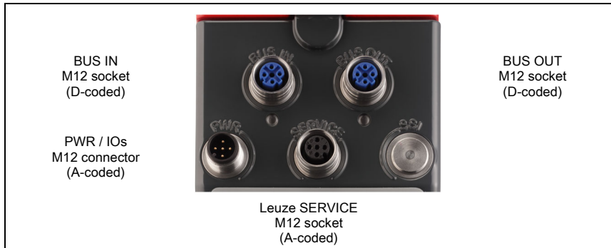
Figure 7.1: Connections of the AMS 358 i
