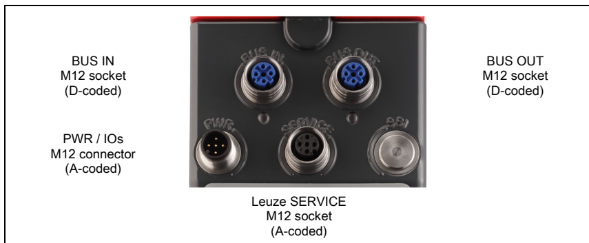
Figure 7.1: Connections of the AMS 338 i
