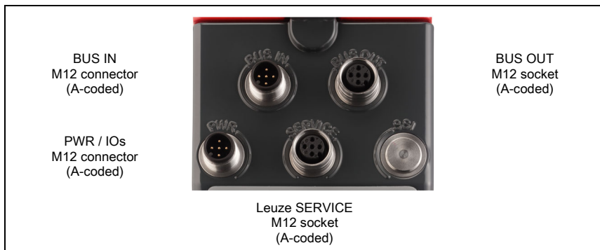
Figure 7.1: Connections of the AMS 335 i
