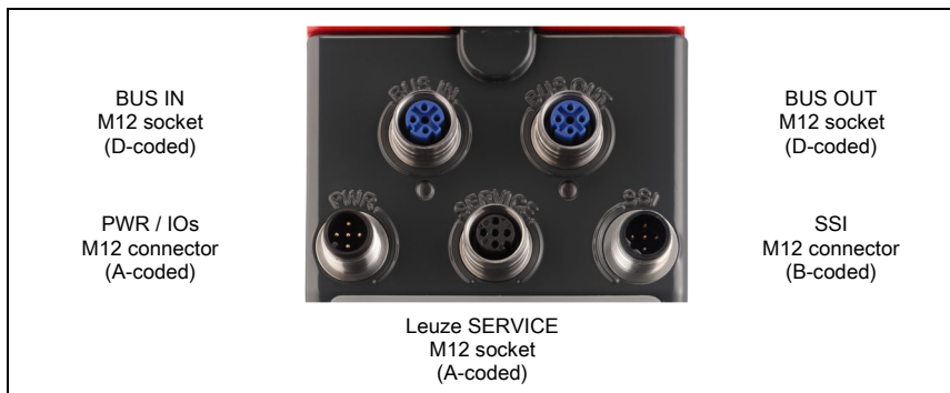
Figure 7.1: Connections of the AMS 348/SSI
