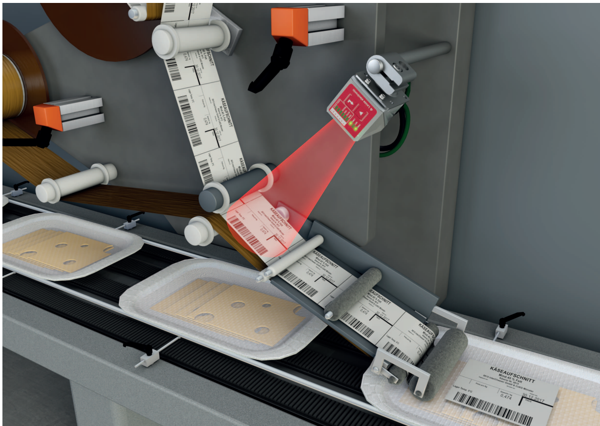
Fig. 5.1: Reading of 1D-codes
