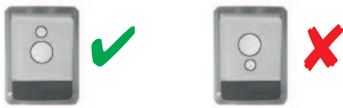
Fig. 6.23: Orientation of the diffuser foil
