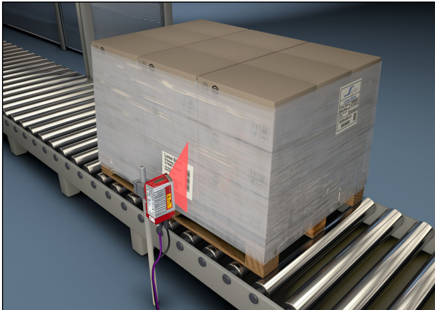
Figure 4.10: Deflection principle for the line scanner
