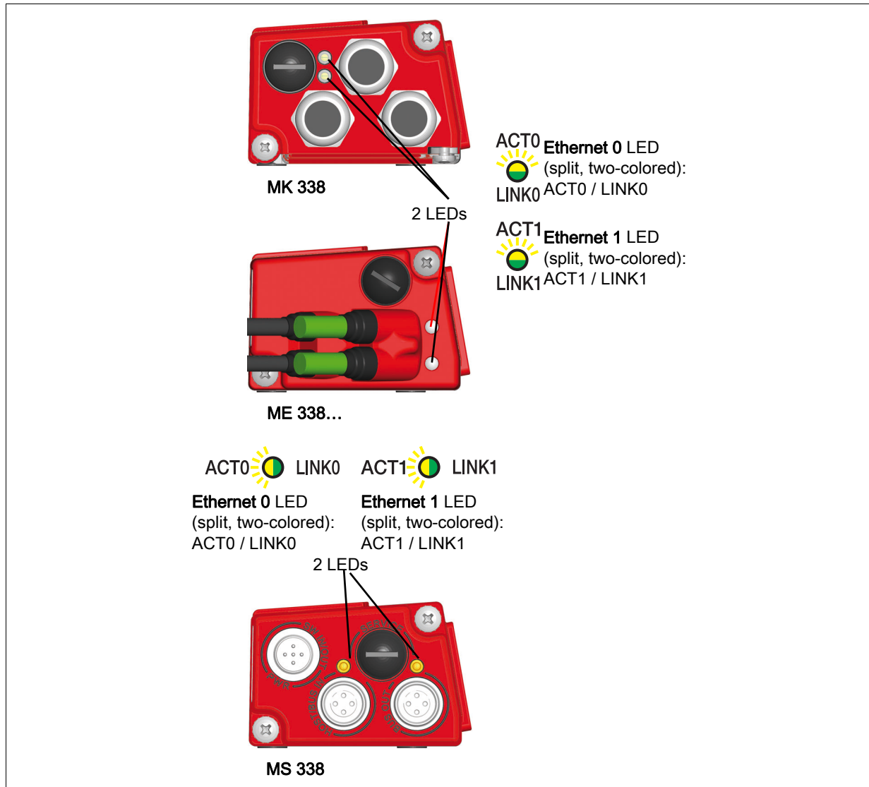
Figure 8.2: MS 338/ME 338.../MK 338 - LED indicators
