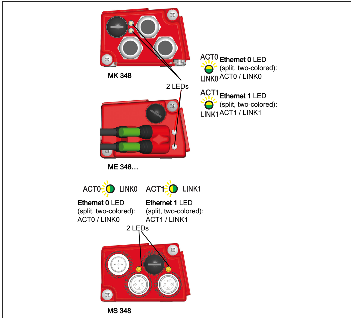
Figure 8.2: MS 348/ME 348.../MK 348 - LED indicators
