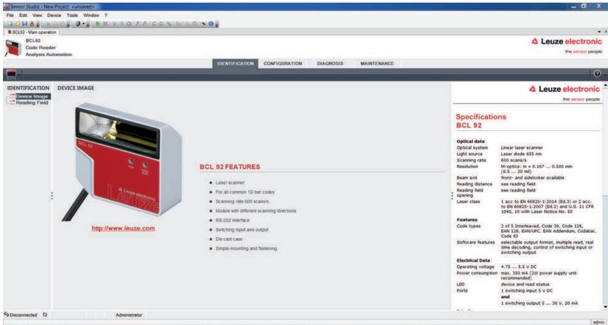
Fig. 6.2: Configuration project: device manager for BCL 92
