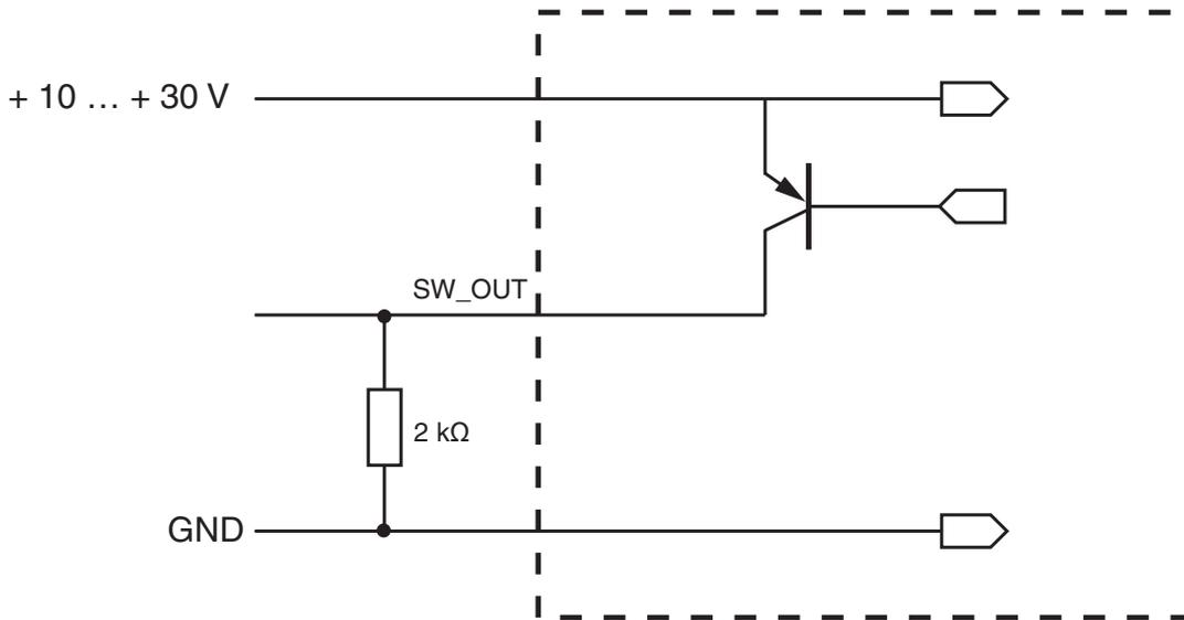
Fig. 5.6: Switching output
