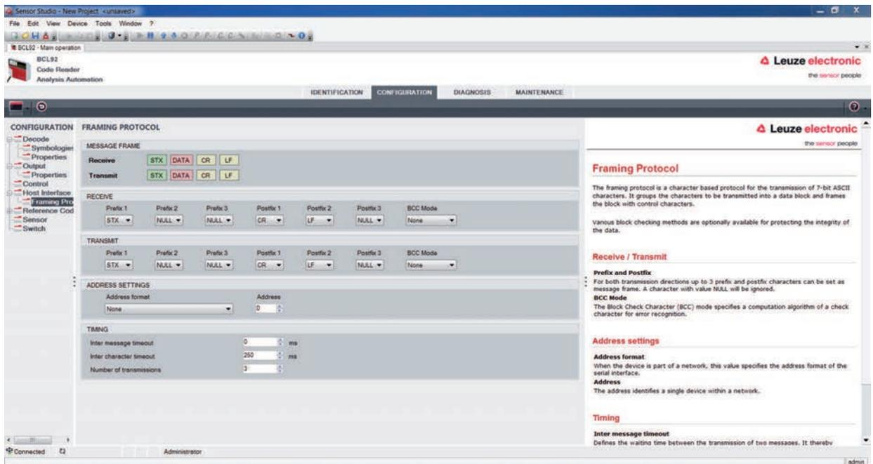
Fig. 6.9: Standard settings of the Properties dialog box (FRAMING PROTOCOL)
