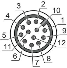
Fig. 5.2: Pin assignment for M12 connector, 12-pin, A-coded
