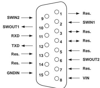
Fig. 5.1: Pin assignment for Sub-D connector, 15-pin
