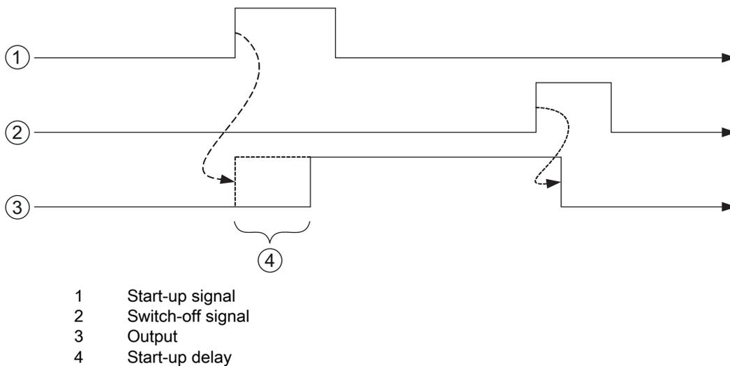
Figure 10.5: Example 1: Start-up delay > 0 and switch-on time = 0
