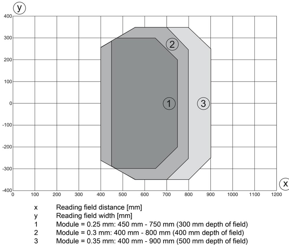
Figure 15.7: Reading field curve - Medium Density
