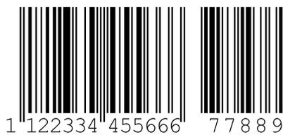
Figure 18.6: Code type 10: EAN 13 Add-on
