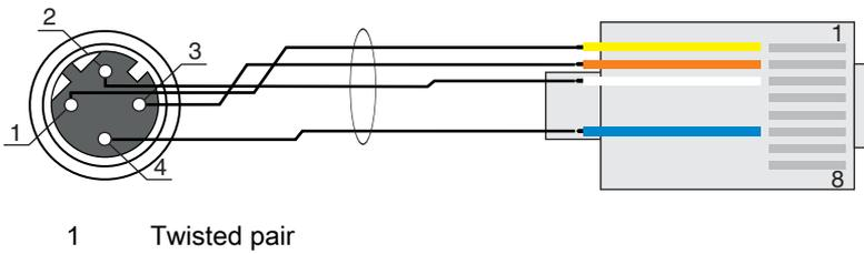
Figure 7.10: HOST / BUS IN cable assignments on RJ-45
