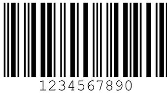
Figure 18.9: Code type 01: Interleaved 2 of 5
