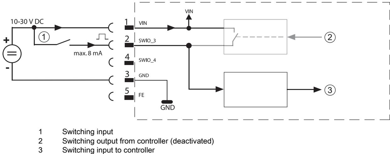
Figure 7.3: Switching input connection diagram SWIO\_3 and SWIO\_4
