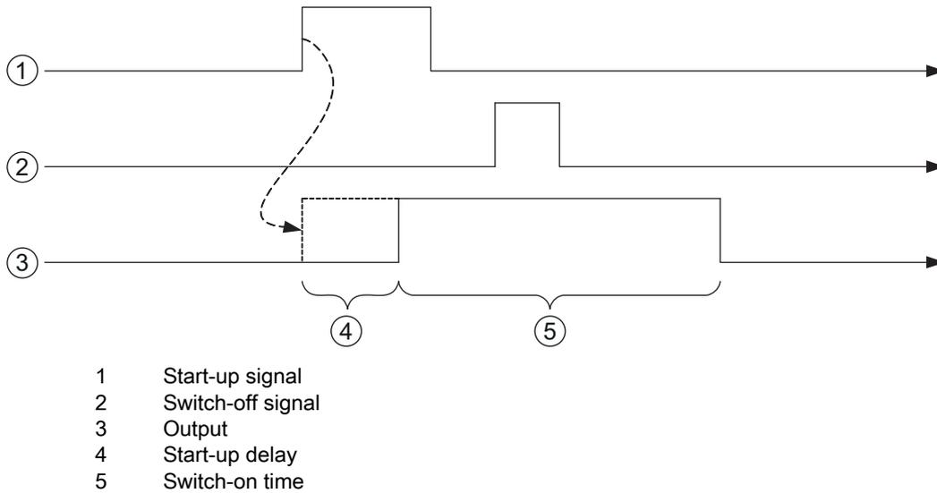
Figure 10.6: Example 2: Start-up delay > 0 and switch-on time > 0
