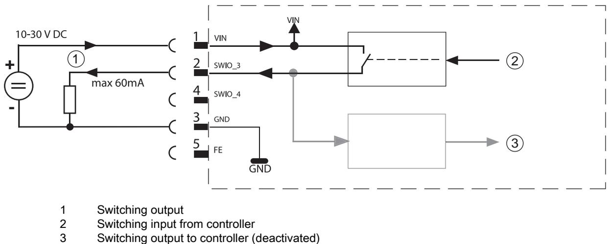
Figure 7.4: Switching output connection diagram SWIO\_3 / SWIO\_4
