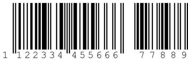
Figure 18.14: Code type 10: EAN 13 Add-on
