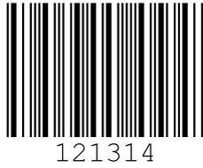
Figure 18.7: Code type 11: Codabar
