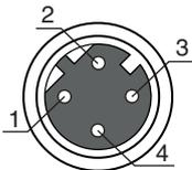
Figure 7.11: M12 socket (D-coded)
