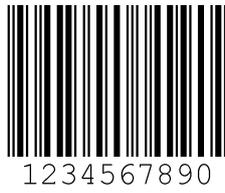
Figure 18.1: Code type 01: Interleaved 2 of 5
