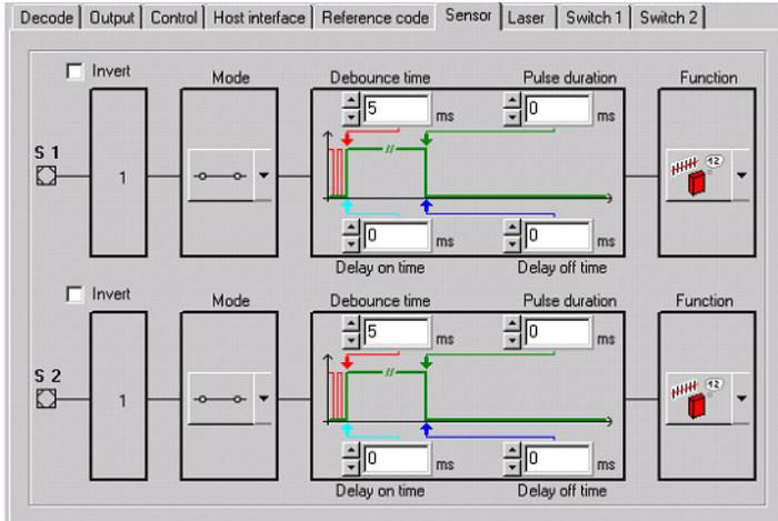
Figure 10.8: Standard setting of the switching input menu
