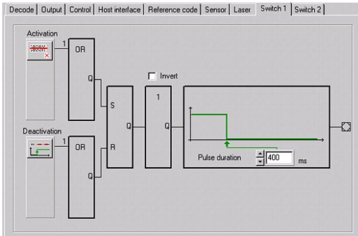
Figure 10.11: Standard setting of the switching output menu
