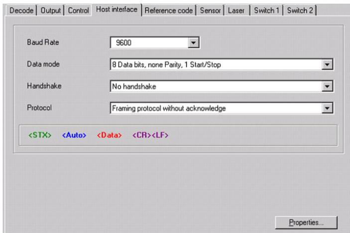
Figure 10.5: Standard setting of the communication menu
