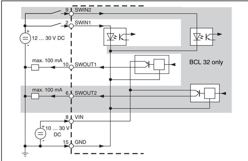
Figure 6.7: Connection diagram switching inputs and outputs BCL 31/32
