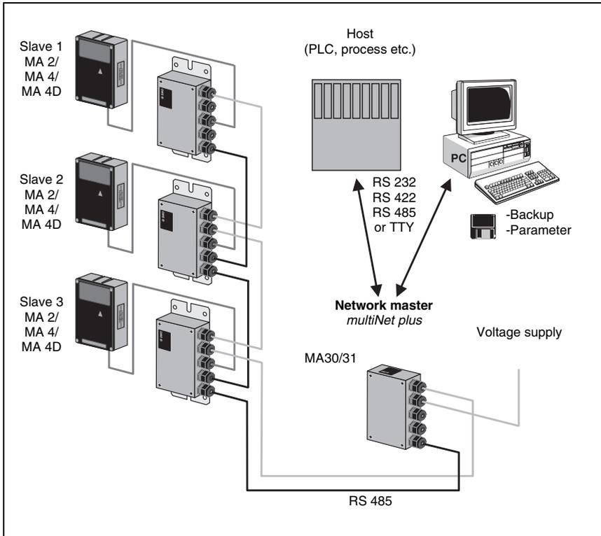
Figure 3.2: Networking possibilities using the multiNet plus (BCL 31)
