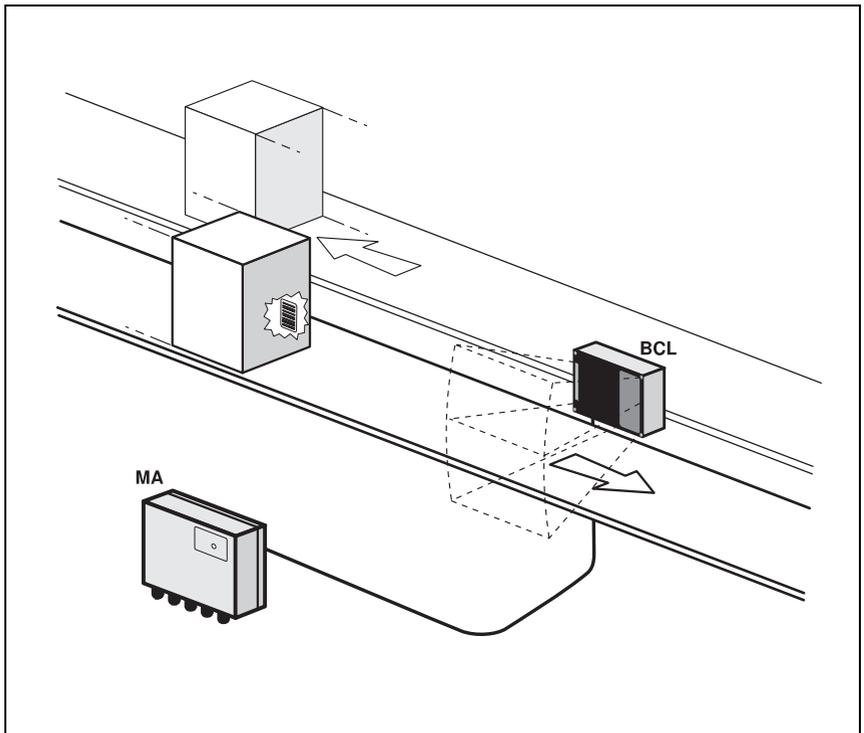
Figure 6.4: Application example "conveyor chain"
