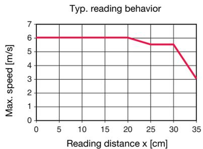
Figure 3.4: Typical reading behavior - RFM 62 read-write unit
