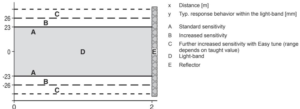
Reference object for detection: 12 mm with TKS 40x60 reflector
