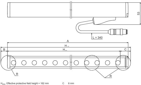
H<sub>PFN</sub> Nominal protective field height = 150 mm
