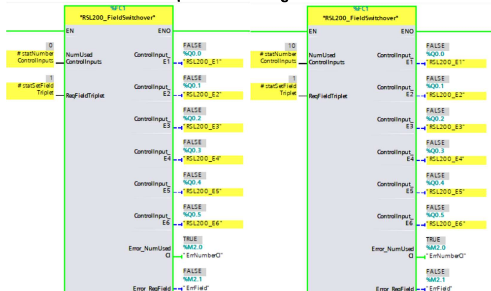
Fig. 3.2: Software function block: NumUsedControlInputs out of range
